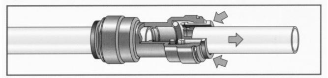
To disconnect, ensure the system is depressurized before removing the tube. Push in collet squarely against face of fitting. With the collet held in this position, the tube can be removed.
