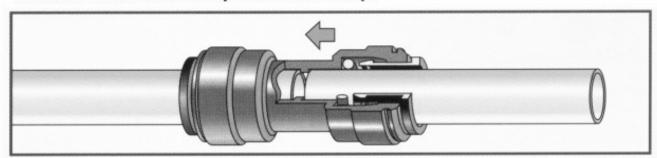
Push the tube into the fitting, to the tube stop. The collet (gripper) has stainless steel teeth which hold the tube firmly in position while the 'O' ring provides a permanent leak proof seal.
