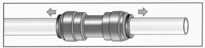
Pull on the tube to check that it is secure. It is a good practice to test the system prior to leaving site and/or before use.
